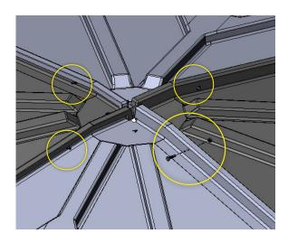
+ When you are bolting the middle hole, you will see two different holes in the metal support bracket. Bolt through the hole that fits best.
