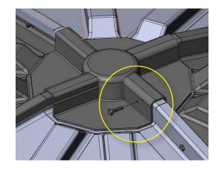
Step 8: You now have a completed 6-Panel Roof. Place roof on top of your constructed wall panels. Be sure the section of roof above the door is flat and does not have a rain guard in the middle.
